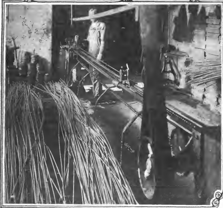
Fig. 1—McCord System of making tubing from long ribbons of sheet brass, at a rapid rate and well, with a seam which adds strength
